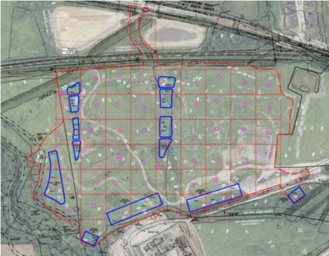
OVERALL TEST PIT LOCATIONS N.T.S.
